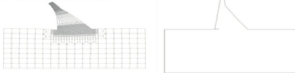
Figure 5-Crack propagation and deformation of Blue stone dam during Kern county earthquake record with massless foundation model ( E_f = 40 \times 10^9 ), cracked area = 3%.
