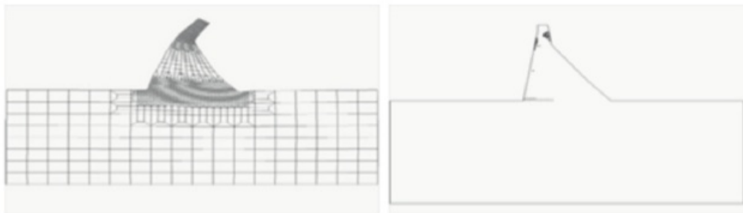
Figure 5-Crack propagation and deformation of Blue stone dam during Kern county earthquake record with massless foundation model ( E_f = 40 \times 10^9 ), cracked area = 3%.
